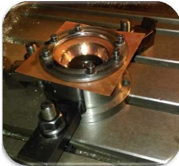
Figure2. A view of the sheet closure in the fixture and deformation of the sheet
