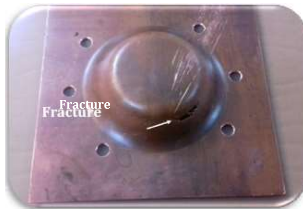
Figure4. A view of rupture after drawing
