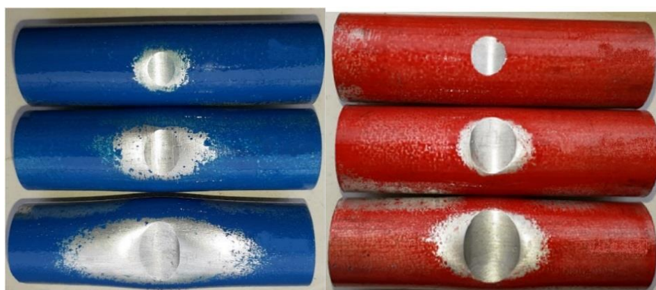
Figure 8. Deformation areas in tubes with an inner diameter of 18 mm, blue color, and tubes with an inner diameter of 12 mm, red color
