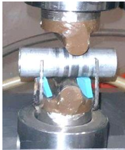
Figure 7. The position of placing the tube between the dies in the press machine
