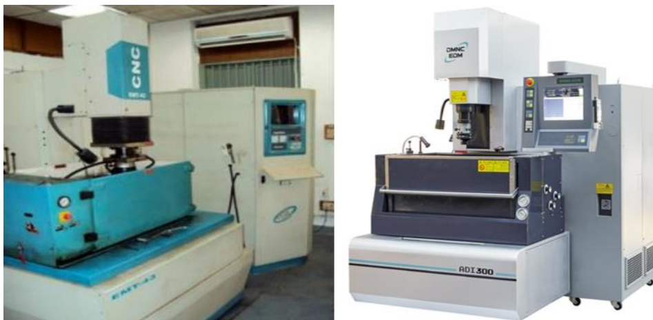
Figure 3. Image of the A30 CNC Die Sinking EDM used in this research
