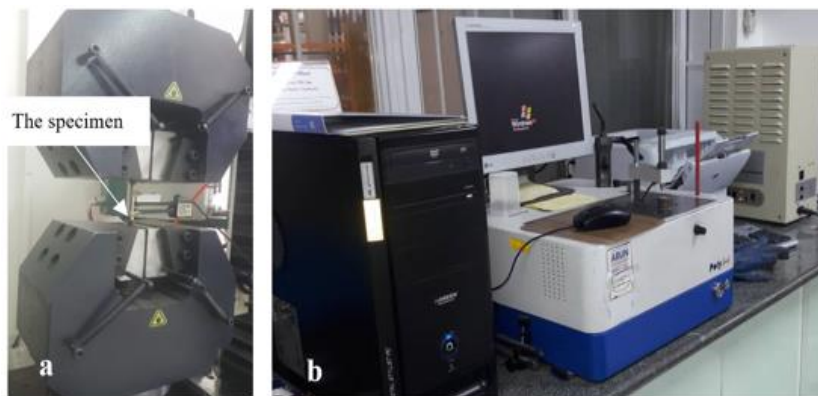
Figure 2. a) The universal test machine STM-250 b) The ARUN technology Poly Spec machine
