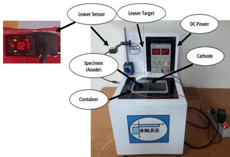
Figure 5. Layer removal setup and measuring the deflection of the specimen using the laser displacement sensor
