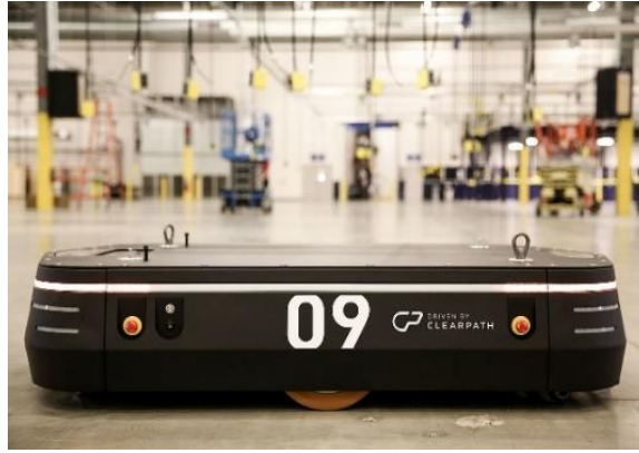
Figure 1. An Industrial mobile robot example: OTTO 1500 self-driving vehicle for heavy-load material transport in warehouses, distribution centers, and factories [1]
