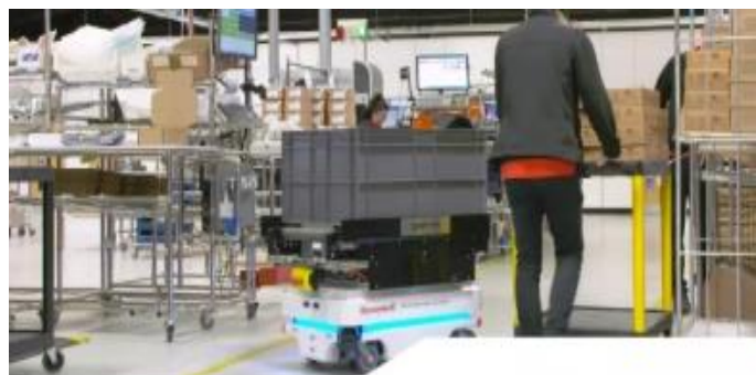
Figure 11. MIR robot Vs anti-collision system for human and other Mir members [40]
