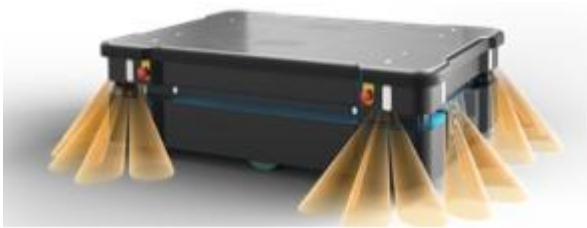
Figure 14. MIR Sensors for proximity detection [42]
