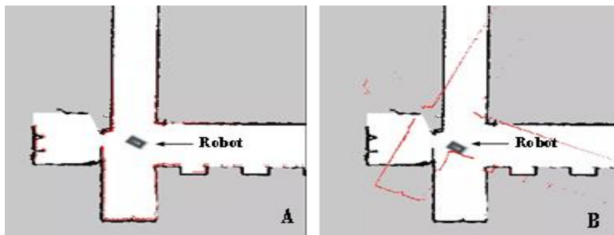
Figure 4. A: Sensor not yet matched to map structure: Sensor matching to map structure [28]
