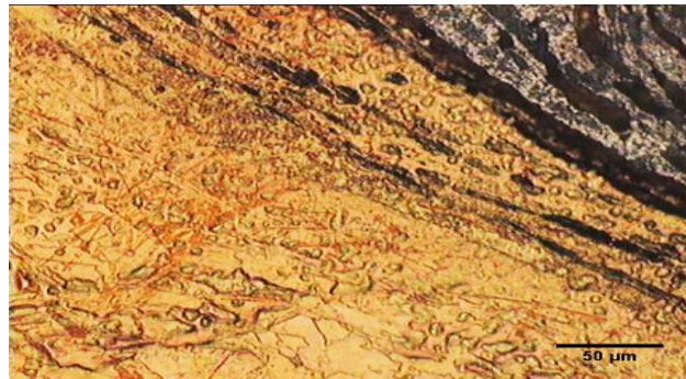
Figure 10. Zone of thermomechanical operations of copper (progressive side)
