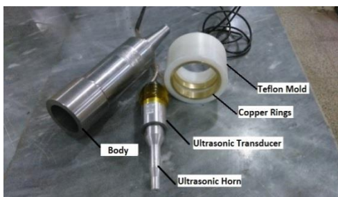
Figure 5. The transducer, copper rings, and tool holder of the vibration setting
