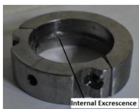
Figure 6. The fixture for clamping the horn
