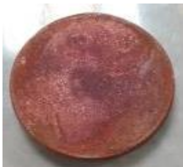
Figure4. Copper sample has been corroded after 20 hours
