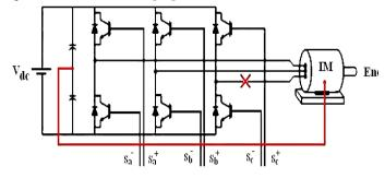
Fig. 5: Scheme of the inverter for faulty machine
