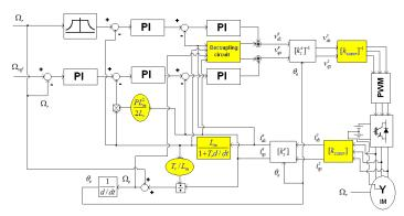
Fig. 4: Block diagram of IRFOC for 3-phase IM drive systems
