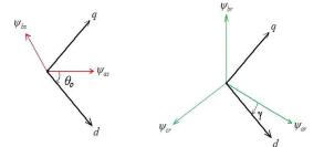
Fig. 2: Stator and rotor winding's flux axes
