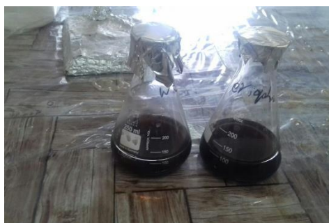
Fig. 2. The color change of the solution obtained by the interaction of the extract and the silver nitrate after 2 hours.
