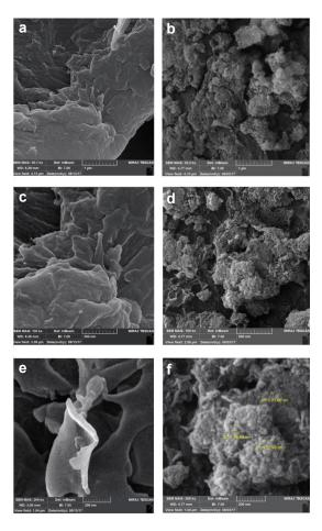
Fig. 5. a. c. e FESEM image of raw sawdust b. d. f  $\rm NiFe_2O_4$  / sawdust nanocomposite.
