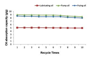
Fig. 8. Oil adsorption capacity of modified sawdust for three types of oil after 10 oil removal cycles.
