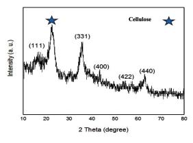
Fig. 3. XRD pattern of NiFe<sub>2</sub>O<sub>4</sub> /Sawdust nanocomposite.
