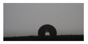
Fig. 2. Optical image of a water droplet on NiFe<sub>2</sub>O<sub>4</sub>/ sawdust nanocomposite.
