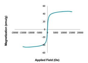
Fig. 6. Hysteresis loop of  $NiFe_2O_4/sawdust$  at room temperature. *Oil-water separation test*
