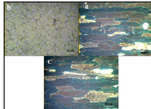
**Fig.8.** Microstructures of the semisolid joints in a) HAZ and b) weld zone and c) base metal
