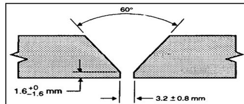
**Fig.2.** Schematic view of the sheets arrangement during the welding
