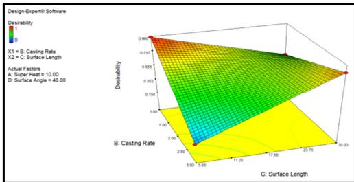
**Fig.6.** 3D desirability diagram of BC interaction factor in maximum sphericity model
