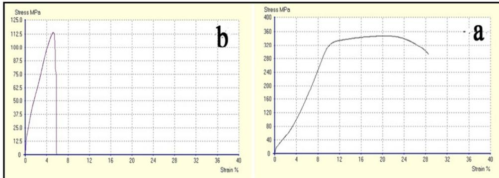
**Fig.10.** Strain-stress diagram of a) non-welded and b) semisolid welded samples
