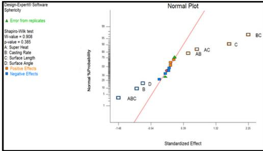
**Fig.4.** Normal plot of effective factors in maximum sphericity
