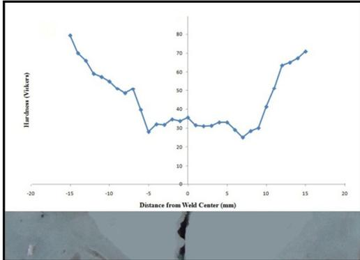
**Fig.9.** Hardness across the cross section of semisolid welded joints (macrograph of the joint after tensile test is also shown.)
