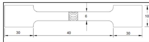
**Fig. 3.** Schematic of the tensile test specimens
