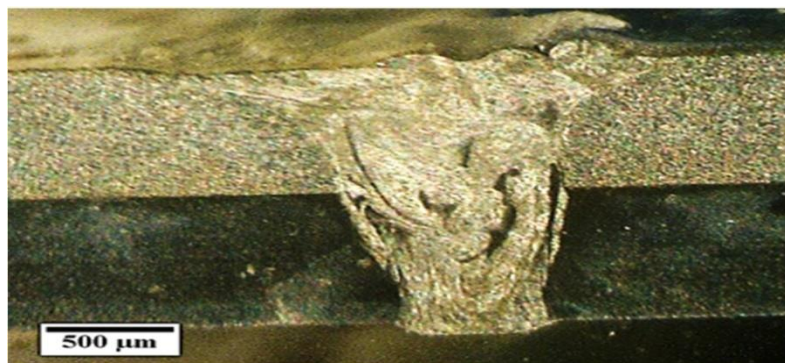
Fig. 4. Macrostructure of a laser weld joint between Inconel 625 and AISI 430 stainless steel.
