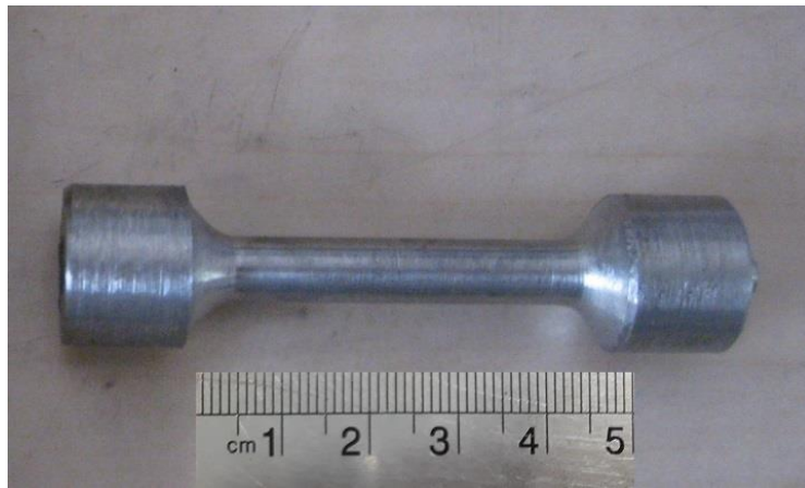
Fig. 5: Sample prepared for creep test.
