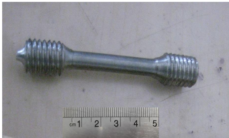
Fig.4. Sample prepared for tensile test.
