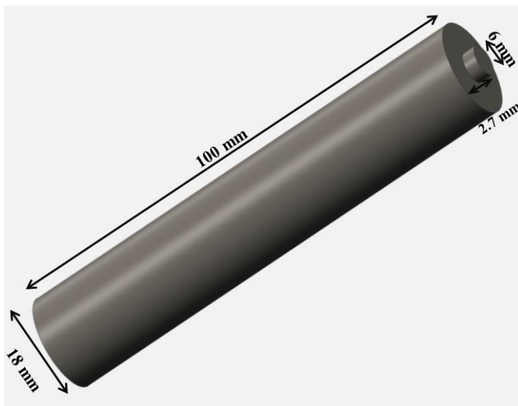
Fig. 1. Dimensions of the tool designed for friction stir welding.
