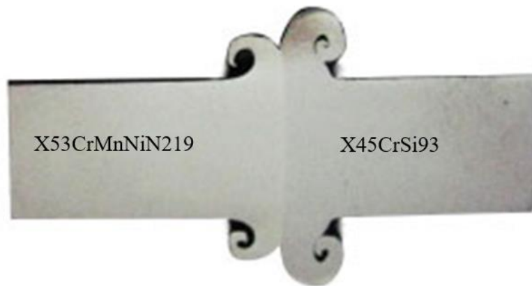
Fig. 4. Schematic longitude section of the joint. Asymmetric flashes can be observed on both sides of the weld interface
