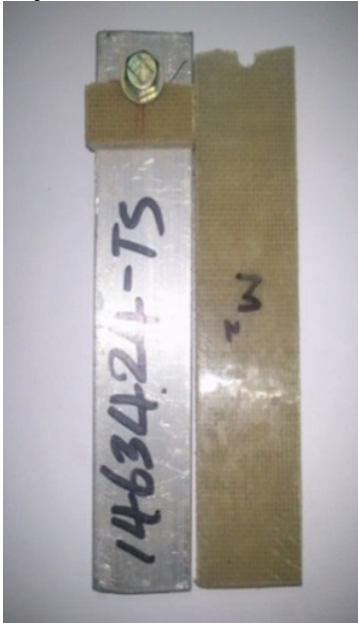
Fig. 12. Joint failed with mechanical fastening
