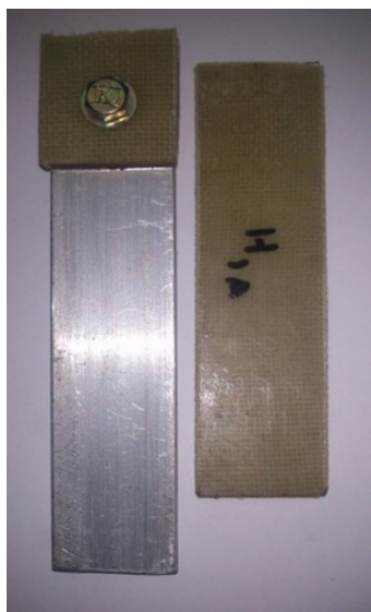
Fig. 14. Joint failed with hybrid joining (Acrylic adhesive)
