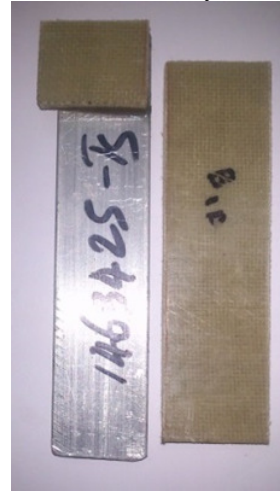
Fig. 8. Joint failed with acrylic adhesive
