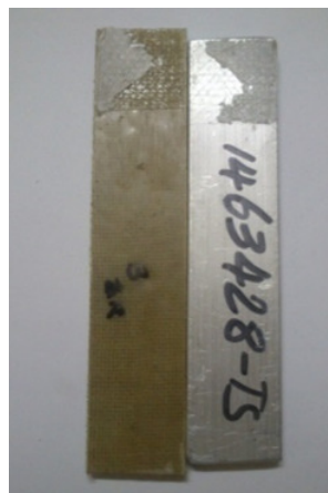
Fig. 10. Joint failed with rubber adhesive
