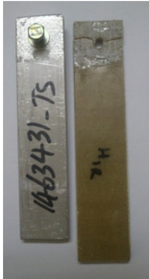
Fig. 16. Joint failed with hybrid joining (rubber adhesive)
