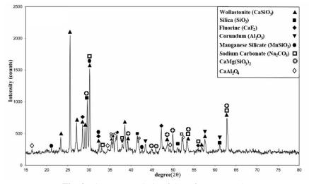
Fig. 2. The XRD analysis of the reference powder
