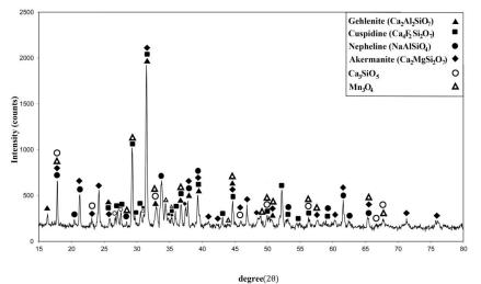
**Fig. 6.** The XRD analysis of sample 1
