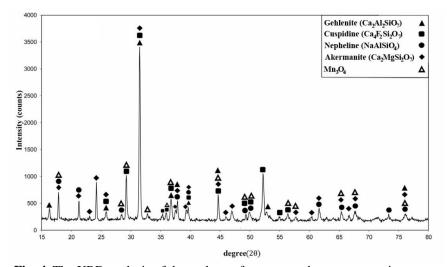
Fig. 4. The XRD analysis of the molten reference powder on groove viscometer
