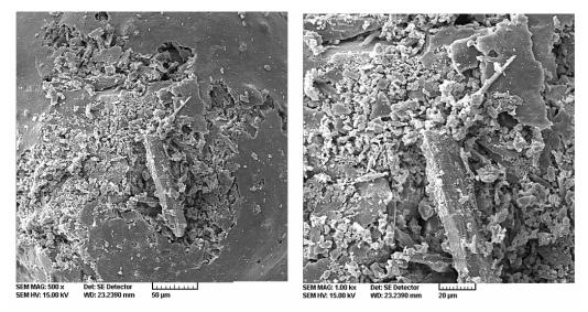
Fig. 3. SEM images of the reference powder(a) 500x (b) 1000x
