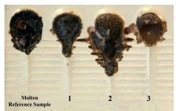
Fig. 1. Schematic illustration of the samples molten on the groove viscometer
