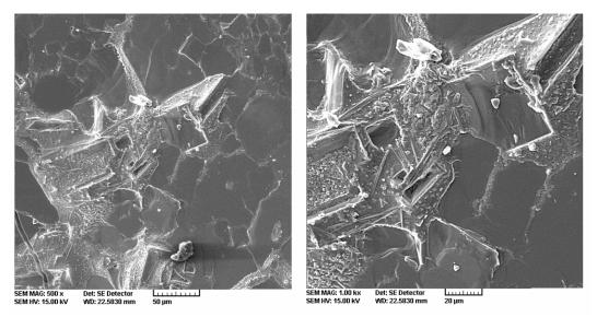
Fig. 5. SEM images of the molten reference powder (a) 500x (b) 1000x
