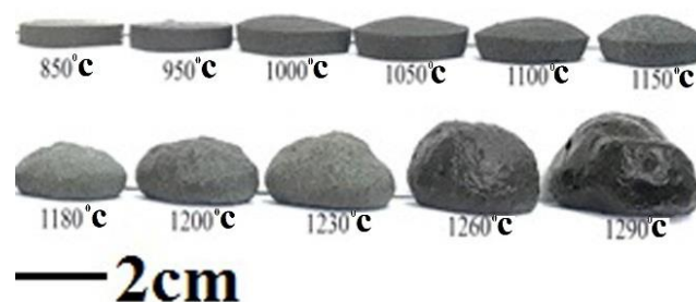
Fig. 10. The appearance of SG50-5SiC sintered at different temperatures.
