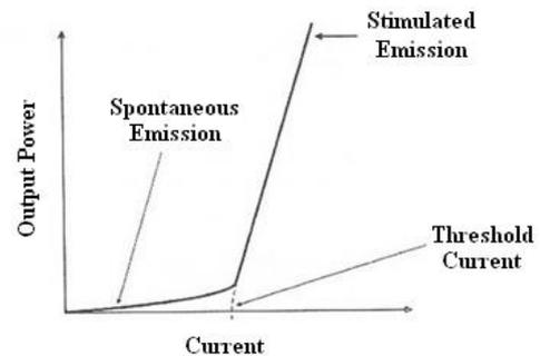
**Fig. 3.** Light output power as a function of current in a LD [3].
