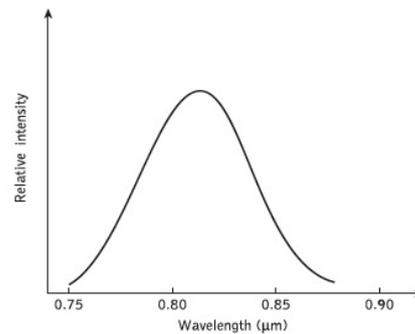
**Fig. 5.** Output spectrum for an AlGaAs surface emitter with doped active region [5].
