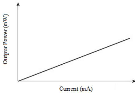
**Fig. 4.** Light output power as a function of current for a LED.
