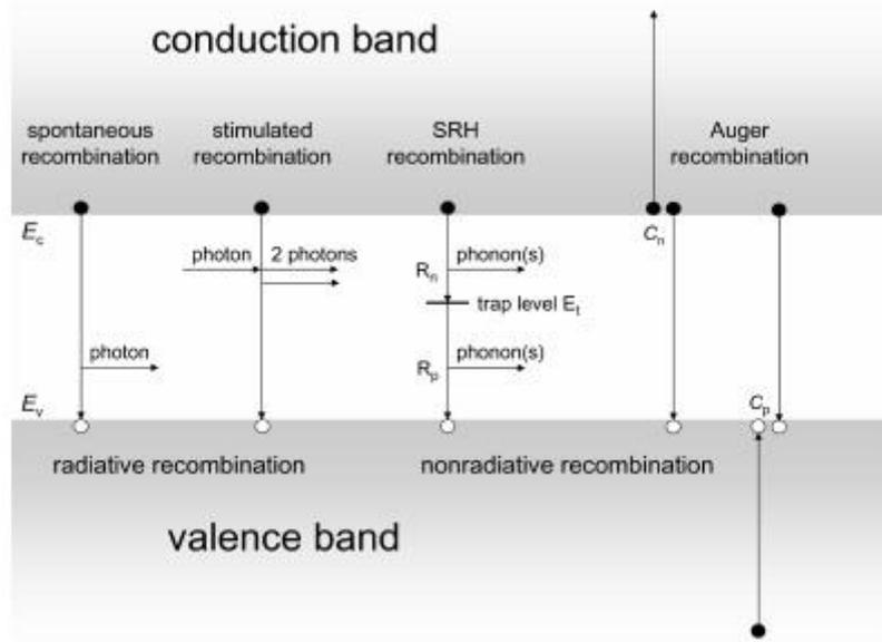
**Fig. 1.** The main mechanisms of electron-hole recombination in semiconductors [1].
