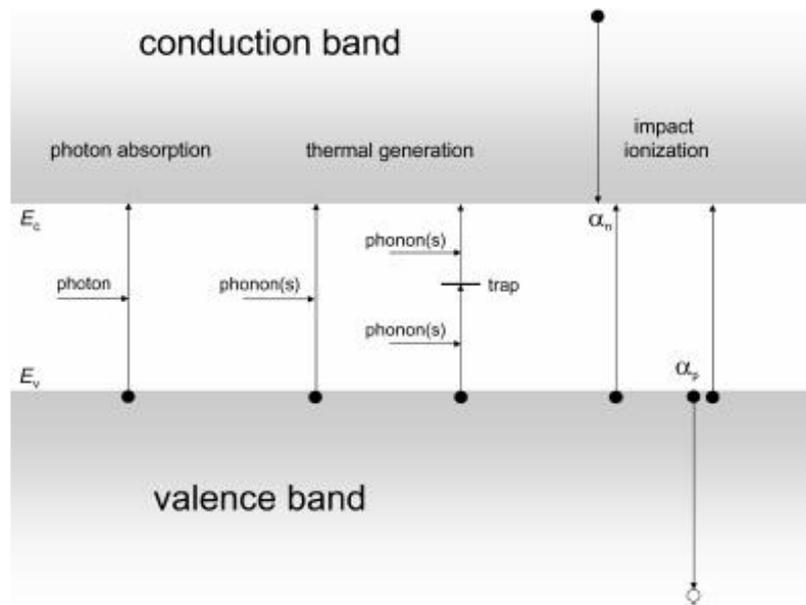
**Fig. 2.** The main mechanisms of electron-hole pair generation in semiconductors [1].
