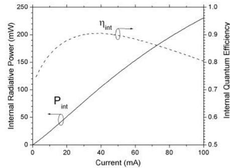
**Fig. 6.** Internal optical power and internal quantum efficiency as a function of current [1].
