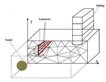
Fig. 1 Configuration of underground blast site
