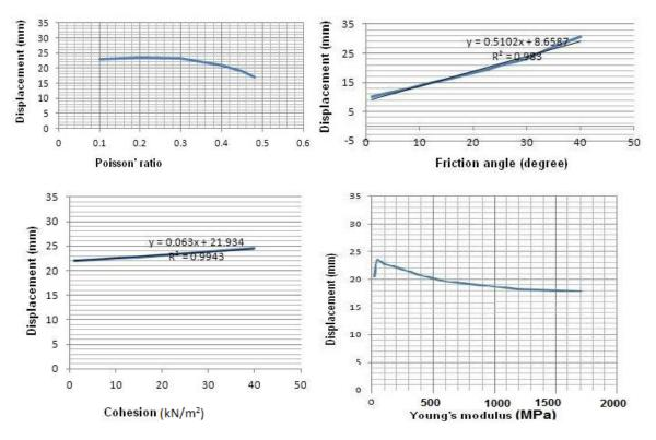
Fig. 5 The relationship between total displacement of the structure foundation and Poisson' ratio, Friction angle, Cohesion and Young's modulus of soil.
