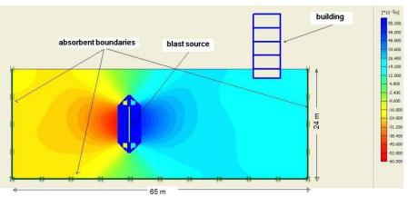
Fig. 2 Structure of the models and soil displacements at 0.25 second
