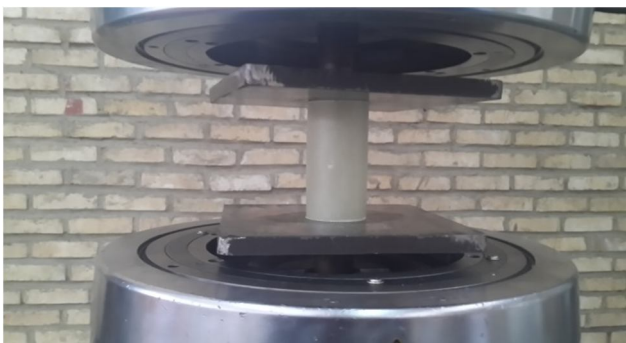
Fig. 4. A circular composite tube during crush test
