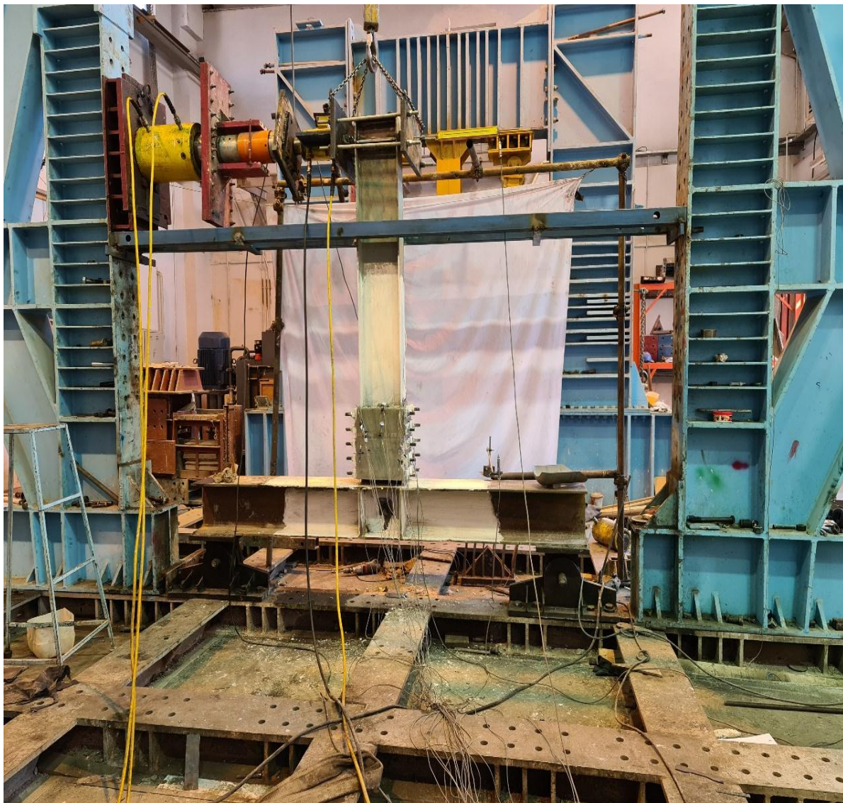
Fig 3.The HS–RBS assembly in the Lab [23]
