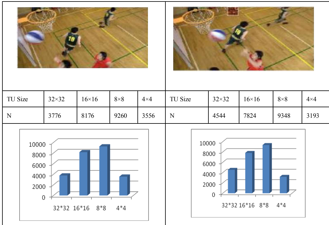
Fig. 2. The sum of histogram differences between two frames
