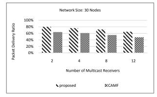
Fig. 13. Packet delivery ratio for a network with 30 nodes and different number of multicast receivers
