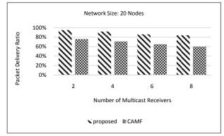
Fig. 12. Packet delivery ratio for a network with 20 nodes and different number of multicast receivers
