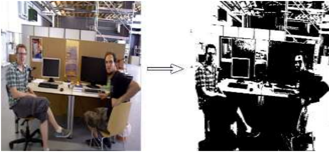
Fig. 2. The pixel value is substituted with the step function
