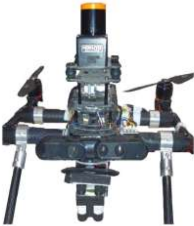
Fig. 6. Our designed UAV: (up) 3D CAD, (down) Assembled UAV equipped with RGBD sensor.
