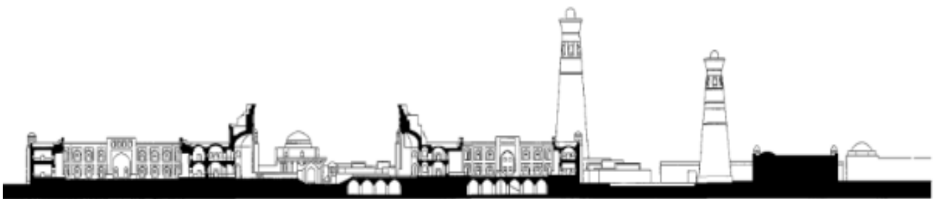
Fig. 3. East-west section through Allah Quli Khan Madrasa (left) and Qutlugh MuradInaq Madrasa, with its underground winter mosque (Herdeg, 1990:53)
