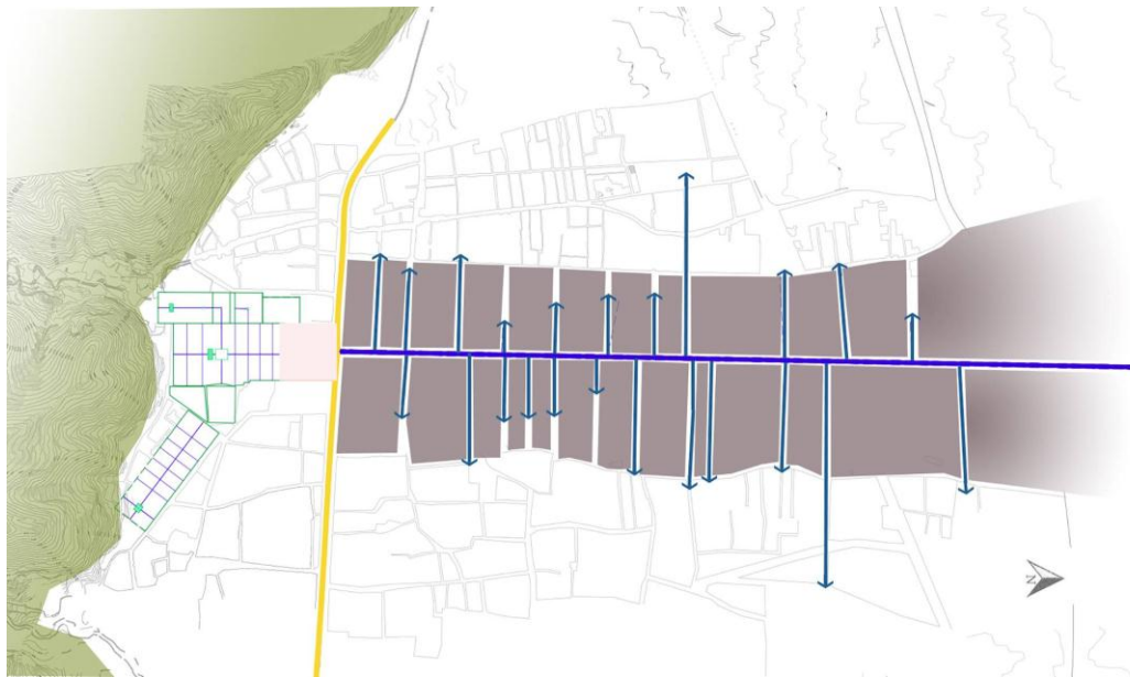
Fig. 4. The effect of the water management system in adaption with the urban access network shaped the geometry of land divisions in the urban landscape of Ashraf al-Belād, based on the comparison of historical documents and the current surveys.
