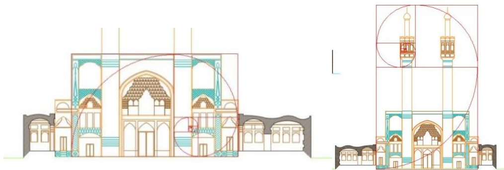
Fig. 9. a) Proportions of the golden spiral in the front view of the Mohammad Shahi entrance (Source: Authors using phi Matrix 1.16 pro software in AutoCAD environment)
