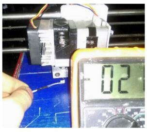
Fig. 2. Object resistance after temperature equilibrium
