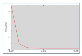
**Fig. 8.** The graph of temperature changes based on time for corner node of upper plate
