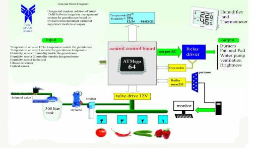
**Fig. 1.** The diagram by using suggested method
