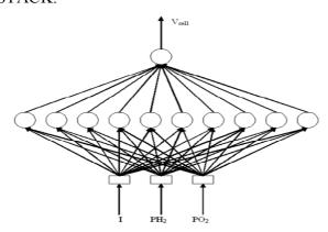
Fig.1.Model of fuel cell NNT
