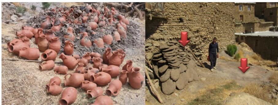
Fig. 8: The stages of pottery production. Placing the pottery and the cow dung (right), and burning cow dung as fuel and the wall of the furnace.
