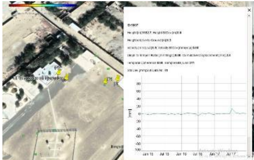
Figure 9. Time series and displacement velocity (in LOS) P3 point are located in near SARAVAN GPS station
