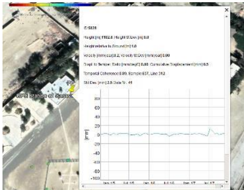
Figure 8. Time series and displacement velocity (in LOS) P2 point are located in near SARAVAN GPS station
