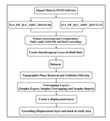
Figure 1. Innovative method: Flowchart of Dinsar data processing
