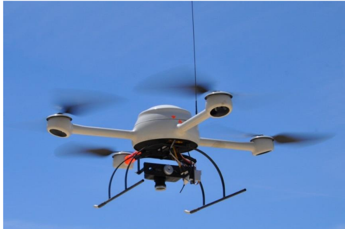
Figure 3. The commercial “ready-to-use” Micro-drones MD 4-200. Payload includes IMU, GPS receiver, downward pointing CIR-modified digital Canon IXUS 100 camera, radio downlink and microprocessor controlled flight control units
