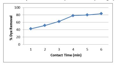
**Fig. 5.** Effect of contact time for 8 ppm erythrosine concentrations; pH 4, 25 °C, agitation rate of 180 rpm and 0.733 g adsorbent in 150 ml of dye solution.
