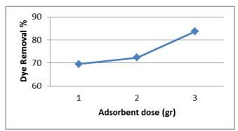
Fig (9): Effect of different copper oxide dose pH 4, 25 °C, agitation rate of 180 rpm and initial dye concentration8mg L<sup>-1</sup> in 150 ml of Erythrosine dye solution.
