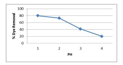
**Fig 4**.Effect of pH on the removal of red carmoisine 25 °C, agitation rate of 180rpm 0.733gr adsorbent in 150 ml of 8 mg L<sup>-1</sup> dye solution
