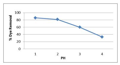
**Fig 3.**Effect of pH on the removal of erythrosine 25 °C, agitation rate of 1800rpm 0.733 gr adsorbent in 100 ml of 8 mg L<sup>-1</sup> dye solution
