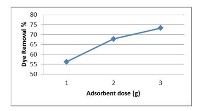
**Fig** (10): Effect of different copper oxide dose pH 4, 25 °C, agitation rate of 180 rpm and initial dye concentration8mg L<sup>-1</sup> in 150 ml of Red Carmoisine dye solution.
