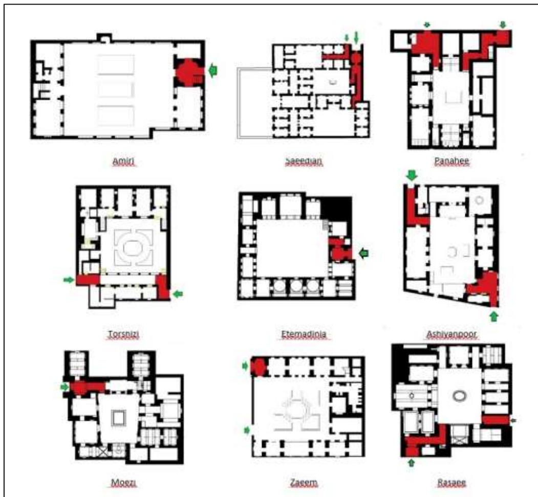
Figure 1: Plan of several sample houses. (Source: Authors). Entrances highlighted with a green arrow and atria highlighted in red
