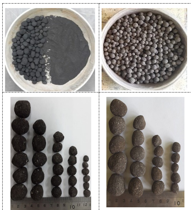
Fig 4. The size distribution of the pellets, before (right) and after (left) of the roasting process
