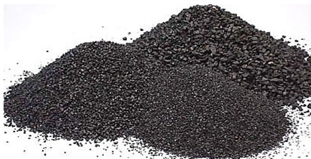
Fig 1. Secondary tailing of iron ore after melting
