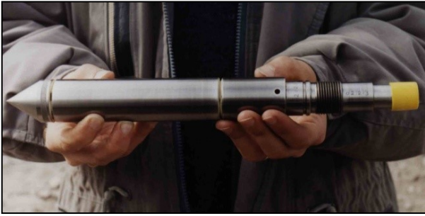
Fig 3. The CPTu cone used in present study
