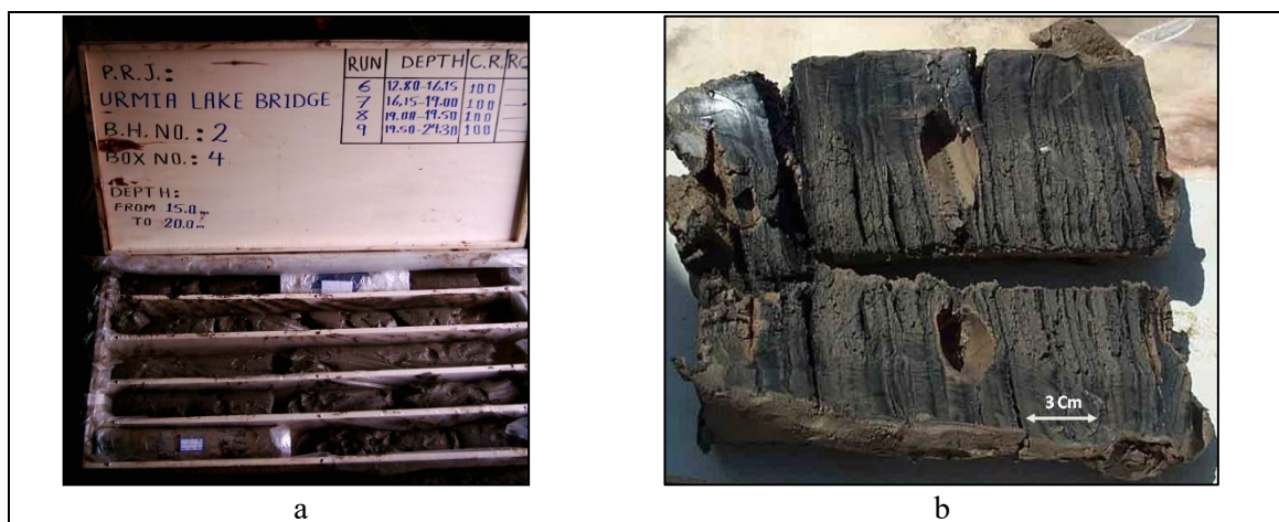
Fig 16. Samples in core box (a), longitudinal cross section of core (b)
