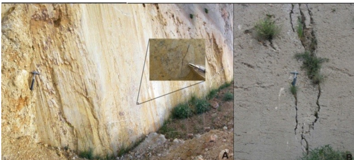
Fig 23. (a) First deformation phase which indicates fractures, major faults, fault joints, filling, and cement in the western Arjan (the observer facing northwest); and (b) Second phase causing young joints (the observer's the northeast).
