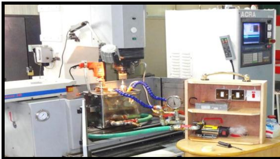
Fig.2 The (CNC) EDM machine with all the fabricated accessories.
