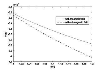
Fig. 5 Circumferential displacement due to centrifugal load at  $\theta = \pi/3$  and  $\omega = 50$  (rad/s) (example 1).
