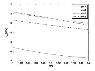
**Fig. 16** Circumferential stress due to centrifugal load and magnetic field along the thickness of FG sphere with various power law indices at  $\theta = \pi/3$  and  $\omega = 50$  (rad/s) (example 3).
