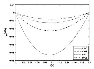
Fig. 15 Shear stress due to centrifugal load and magnetic fieldalong the thickness of FG sphere with various power law indices at  $\theta = \pi/3$  and  $\omega = 50$  (rad/s) (example 3).
