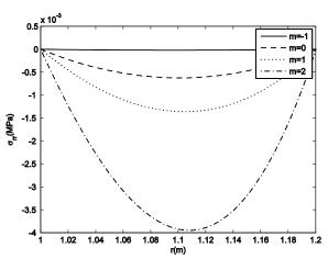
**Fig. 14** Radial stress due to centrifugal load and magnetic field along the thickness of FG sphere with various power law indices at  $\theta = \pi/3$  and  $\omega = 50$  (rad/s) (example 3).
