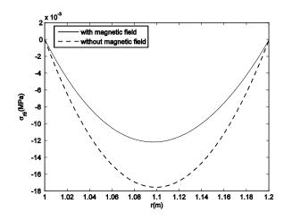
**Fig. 4** Shear stress due to centrifugal load at  $\theta = \pi/3$  and  $\omega = 50$  (rad/s) (example 1).
