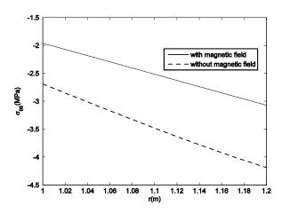
**Fig. 6** Circumferential stress due to centrifugal load at  $\theta = \pi/3$  and  $\omega = 50$  (rad/s) (example 1).
