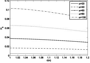
**Fig. 12** Perturbation due to various angular velocities at  $\theta = \pi/3$  (example 2).
