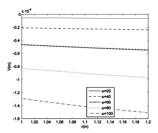
Fig. 8 Circumferential displacement due to magnetic field and various angular velocities at  $\theta = \pi/3$  (example 2).
