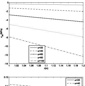
Fig. 11 Circumferential stress due to magnetic field and various angular velocities at  $\theta = \pi/3$  (example 2).
