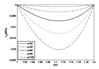
**Fig. 9** Radial stress due to magnetic field and various angular velocities at  $\theta = \pi/3$  (example 2).
