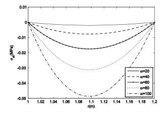
**Fig. 10** Shear stress due to magnetic field and various angular velocities at  $\theta = \pi/3$  (example 2).
