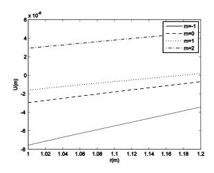
**Fig. 13** Radial displacement due to centrifugal load and magnetic fieldalong the thickness of FG sphere with various power law indices at  $\theta = \pi/3$  and  $\omega = 50$  (rad/s) (example 3).
