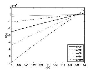
**Fig. 7** Radial displacement due to magnetic field and various angular velocities at  $\theta = \pi/3$  (example 2).
