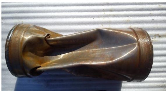
Fig.13 Model test after collapse.
