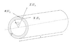
**Fig. 1** Geometry of a cylindrical shell.
