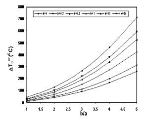
**Fig. 11** Variation of the buckling critical temperature gradient vs. b/a for different FGRP with linear thickness change in y direction under non-linear temperature rise across the thickness ( $c_1$ ,  $c_2$ =const.).
