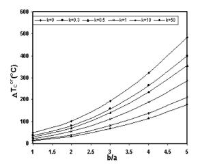
**Fig. 10** Variation of the buckling critical temperature gradient vs. b/a for different FGRP with linear thickness change in x direction under non-linear temperature rise across the thickness ( $c_1$ ,  $c_2$ =const.).
