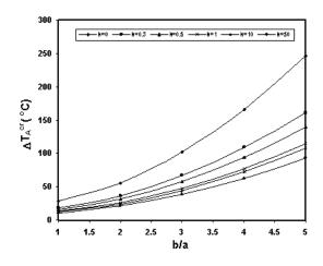
**Fig.2** Variation of buckling critical temperature gradient vs. b/a for different FGRP with linear thickness change in x direction under uniform temperature rise ( $c_1$ ,  $c_2$  =const.).
