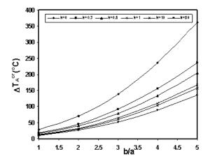
Fig.3 Variation of buckling critical temperature gradient vs. b/a for different FGRP with linear thickness change in y direction under uniform temperature rise ( $c_1$ ,  $c_2$  =const.).
