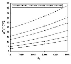
Fig. 12 Variation of the buckling critical temperature gradient vs.  $c_1$  for different FGRP with linear thickness change in x and y directions under non-linear temperature change across the thickness (b/a = 1,  $c_2 = \text{const.}$ ).
