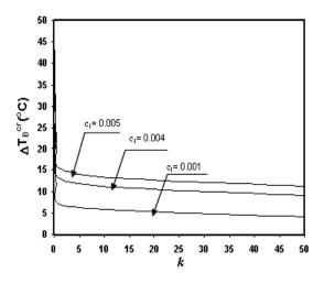
Fig. 9 Variation of the buckling critical temperature gradient vs. material index k for different FGRP with linear thickness change in both x and y directions under linear temperature across thickness (b/a = 1).
