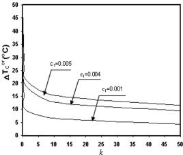
Variation of the buckling critical temperature gradient vs. material index k for different FGRP with linear thickness change in both x and y directions under non-linear temperature across thickness (b/a = 1).
