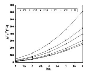
Fig. 7 Variation of the buckling critical temperature gradient vs. b/a for different FGRP with linear thickness change in y direction under linear temperature change across the thickness ( $c_1$ ,  $c_2$ =const.).
