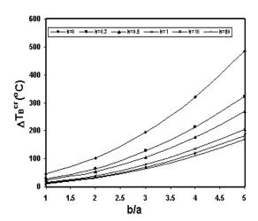
Fig. 6 Variation of the buckling critical temperature gradient vs. b/a for different FGRP with linear thickness change in x direction under linear temperature change across the thickness ( $c_1$ ,  $c_2$ =const.).
