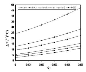
Fig. 8 Variation of the buckling critical temperature gradient vs.  $c_1$  for different FGRP with linear thickness change in x and y directions under linear temperature change across the thickness (b/a=1,  $c_2=$ const.).
