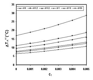
**Fig.4** Variation of buckling critical temperature gradient vs.  $c_1$  for different FGRP with linear thickness change in both x and y directions and under uniform temperature rise  $(b/a = 1, c_2 = \text{const.})$ .
