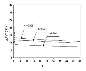
Fig. 5 Variation of the buckling critical temperature gradient vs. material index k for different FGRP with linear thickness change in both x and y directions under uniform temperature rise (b/a = 1,  $c_2 = const.$ ).
