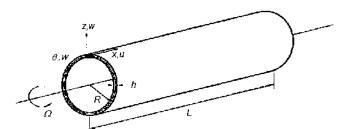
Fig. 1 Spinning cylindrical shell, geometry and coordinates.
