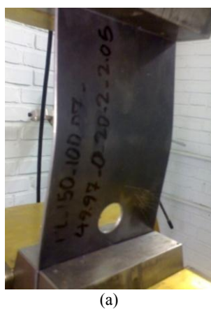
Fig.16 Specimens with circular cutouts under experimental buckling tests: (a) pl-150-100.07-49.97-0-20.2-2.1 specimen. (b) pl-210-100-49.6-26.3-20.2-2.1 specimen.
