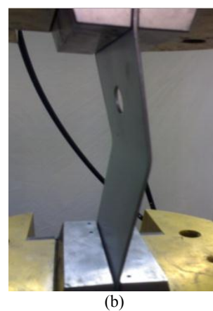
Fig.16 Specimens with circular cutouts under experimental buckling tests: (a) pl-150-100.07-49.97-0-20.2-2.1 specimen. (b) pl-210-100-49.6-26.3-20.2-2.1 specimen.
