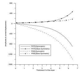
**Fig. 7** Variation of amplitude of normal displacement.
